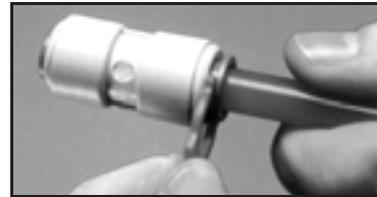
Insert the locking clip. The locking clip secures the collet in its position to prevent an accidental disconnection of the tube.
